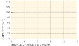
Trickle charge test at +45°C of Ni-MH Button Cells (trickle charge at 0.03 CA)
